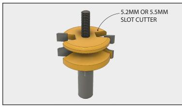
Place the 5.2mm or 5.5mm slot cutter on the bit's arbor, followed by the remaining components (the shims, bearings, washers and nut). Tighten the nut with the wrench or pliers.
