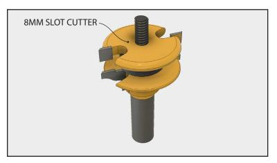
Place the 8mm slot cutter on the bit's arbor and stack the shims, bearing, washer and nut on top. Tighten the nut with the wrench or pliers.
