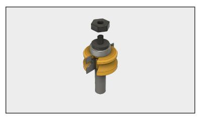
Wrap a rag around the router bit to protect your hand and provide a solid grip. Loosen the nut at the top of the bit with a wrench or pliers.
