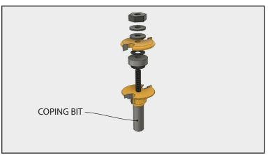
Grip the coping bit with a rag to protect your hands and loosen the nut with a wrench or pliers. Remove the nut,
